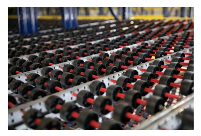
Carton flow is a form of shelving that uses a gravity that rotates products on a first in-first out inventory cycle. Product is loaded on one side and picked up on the opposite in which the next load automatically moves forward. It provides proper circulation and fast access of materials. It used for low volume case picking
